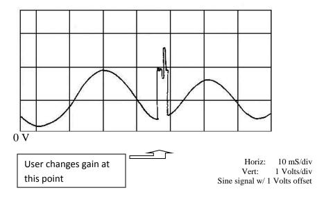
If you notice the zero level of the output has drifted (as maybe seen in the first few minutes after the amplifier is turned on) you can invoke the self-trimming feature by changing the gain, or by just double-clicking the Gain button.
